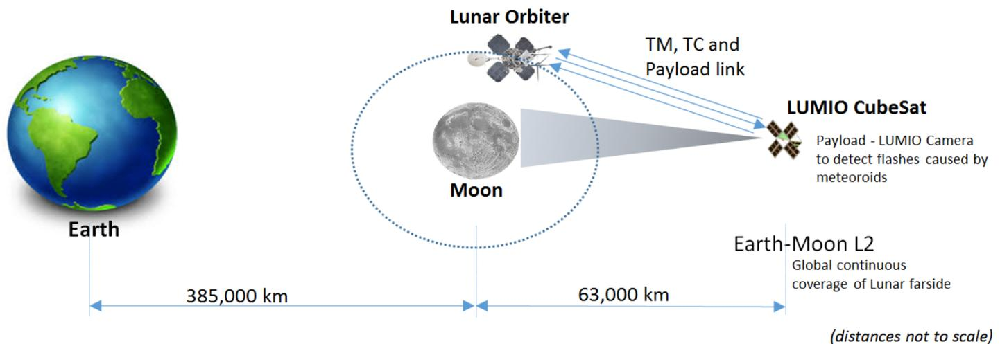
**Lunar Meteoroid Impacts Observer (LUMIO)** is a 12U CubeSat mission to a halo orbit at Earth-Moon L2 that shall observe, quantify, and characterize meteoroid impacts on the Lunar farside by detecting their impact flashes, complementing Earth-based observations on the Lunar nearside, to provide global information on the Lunar Meteoroid Environment and contribute to Lunar Situational Awareness.
